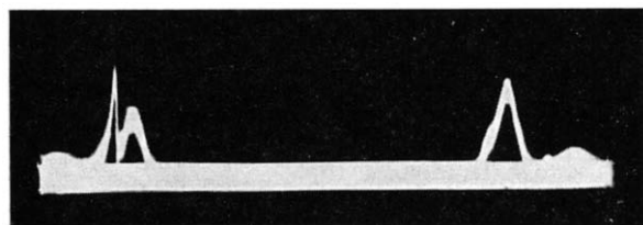
Fig. 1. Electrophoretic pattern of the unfractionated proteins. pH = 8.5, ionic strength 0.057 (Michaelis buffer).
