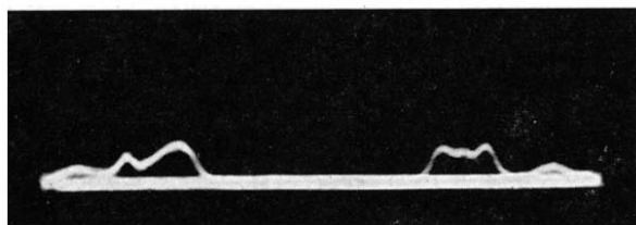
Fig. 2. Electrophoretic pattern of the protein containing less of the slowest fraction. pH = 8.3, ionic strength 0.1.
